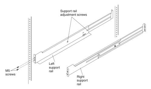
Figure 15. Installing the support rails
